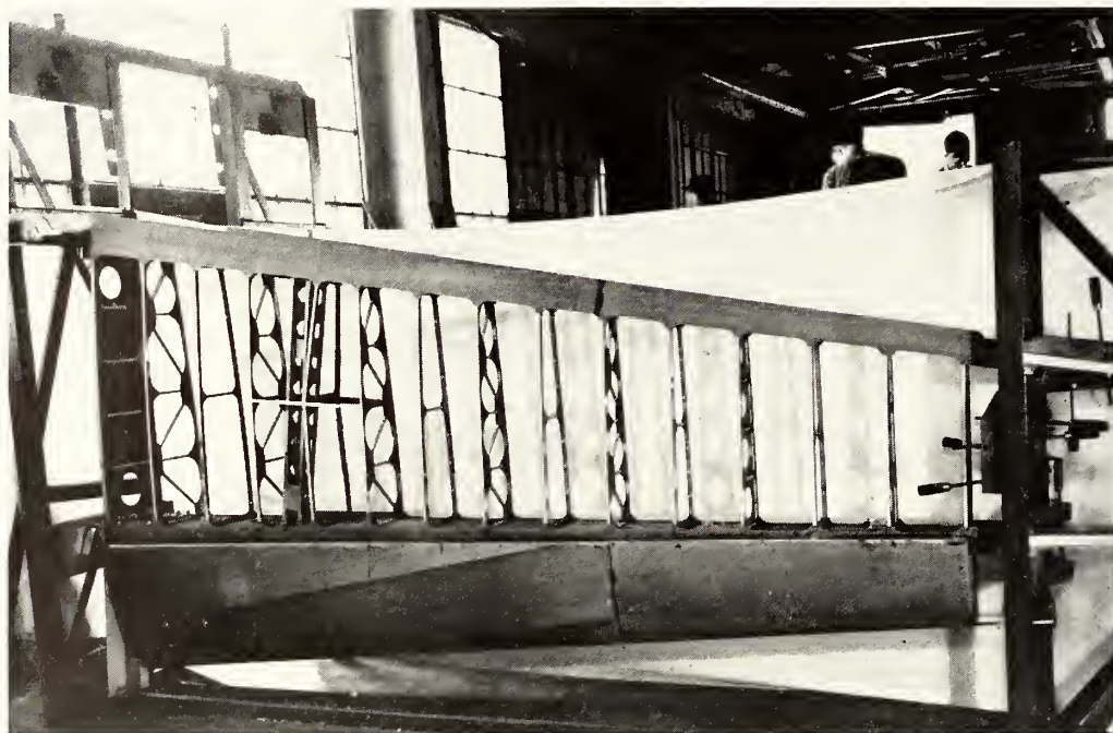
FIGURE 5-51.—Ribs in place between front and rear spars of wing section.
